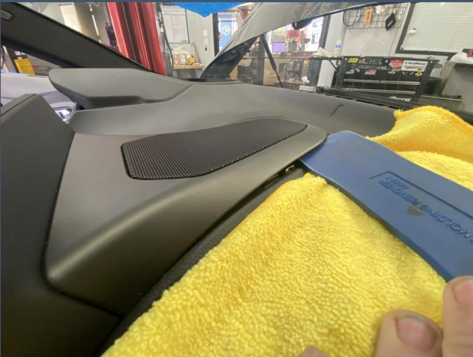
Pry up on a leading edge until you can get your fingers under the panel and apply more grip to pull up. (This grill is snap fit and no fasteners are holding it in place)
