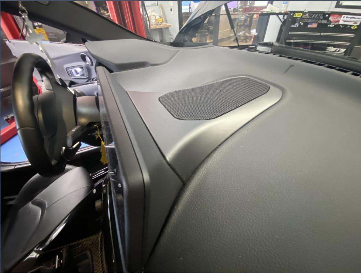
Then start by removing the center speaker grill from the dash. This is not a easy part to remove, it will take some force.
