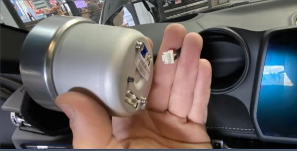
Now if installing your gauge, feed your wire through the opening and connect to the gauge, then slip your gauge in the pod, **use the supplied square "O" ring if needed.** This will be a friction fit. (Depending on the brand of your gauge)
