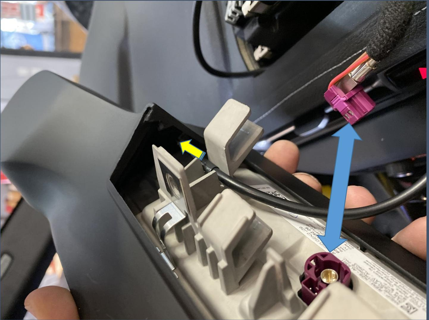
Now reinstall the screen connector, and if needed run the connection wires or lines through the gauge pods opening to the cup. This can be done afterwards if needed as the opening is ample. Then snap the assembly back on to the dash, make sure the clips shown previously by green arrows are secure in the dash.
