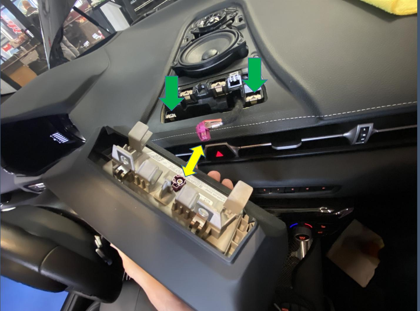
The screen is now free to take out of the car and on to a clean dry bench or work place.
