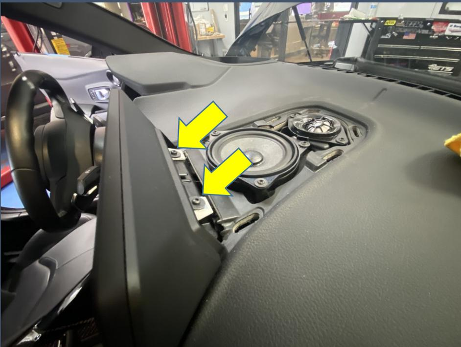
You will find 2 screws, these will require a (T20) Torx bit, remove both screws.
