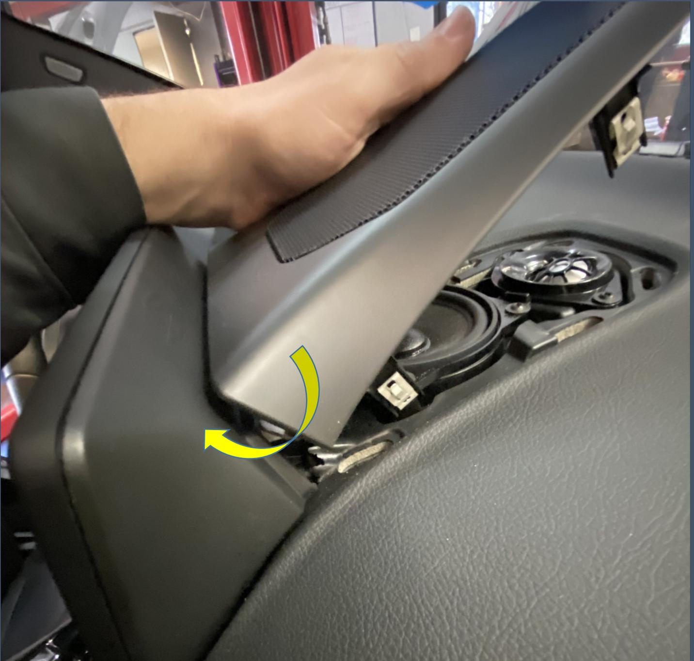
Remember to hook the front tabs in before snapping in the clips!
