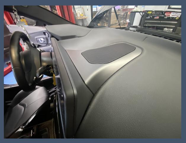
Then start by removing the center speaker grill from the dash. This is not a easy part to remove, it will take some force.
