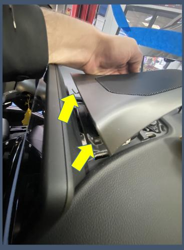
Be careful when lifting off the dash as there are 2 hook shaped metal tabs that go under the screen bezel you will have to tip it up, out and forward in one movement.
