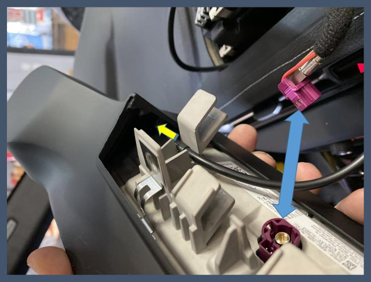
Now reinstall the screen connector, and if needed run the connection wires or lines though the gauge pods opening to the cup. This can be done afterwards if needed as the opening is
