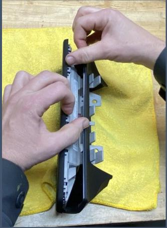
With the rear cover (bezel) removed, the new PodWurX gauge pod can be snapped in to its place.
