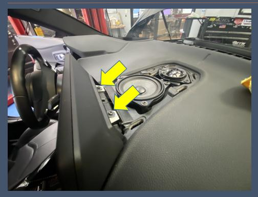
You will find 2 screws, these will require a (T20) Torx bit, remove both screws.
