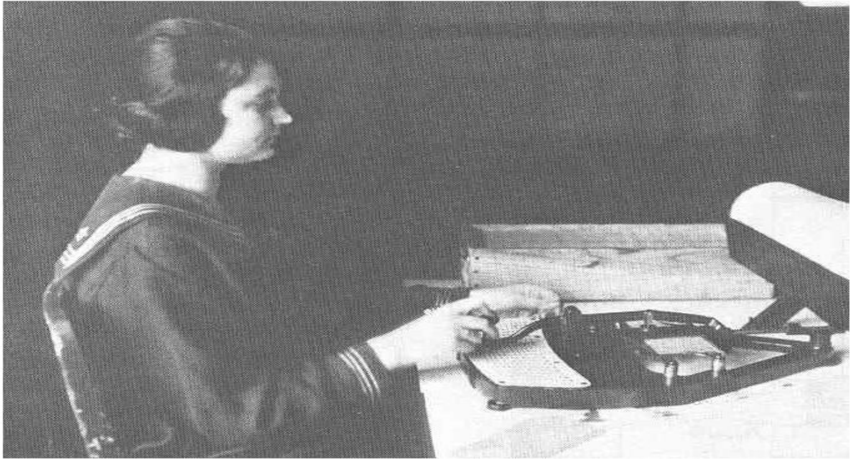
Above: The Pantographic card punch in operation. The operator holds the stylus over the template. The card is in the punch station above the template. Photo (from the 1920 census): [44] .
