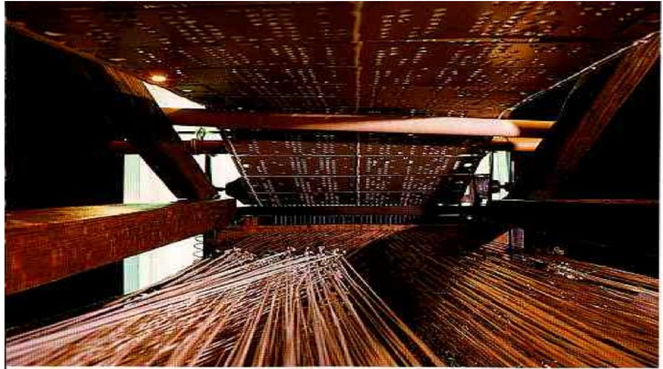
Jacquard's Loom showing the threads and the punched cards
