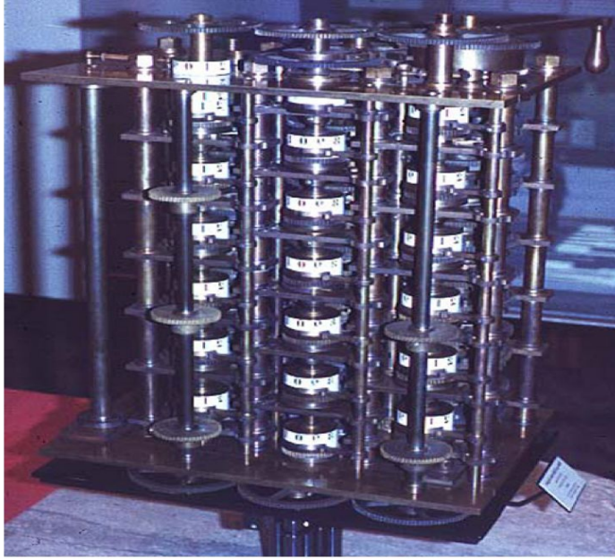
A small section of the type of mechanism employed in Babbage's Difference Engine [photo © 2002 IEEE]
