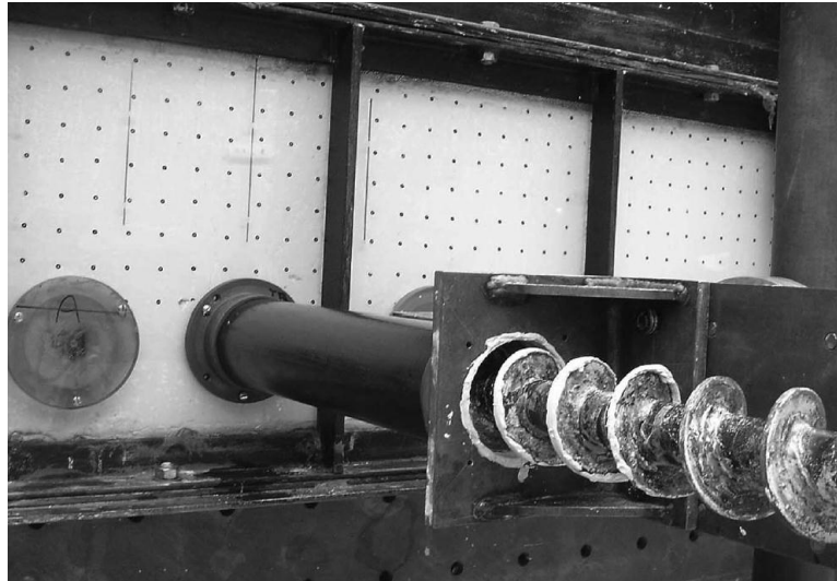
Figure 2-1. The front Perspex window showing maker beads and tunnelling device (Fig. 3 in Chapman et al. [2007])
