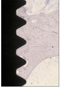
**Fig 4** Survey appearance from a ground section representing a titanium implant 1 month after placement in rabbit cortical bone. The diameter of the implant is 3.75 mm and the total length is 8 mm. The distance between the thread peaks is 600 µm. Periosteal and endosteal new bone formation is clearly visible.
