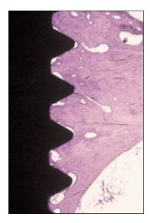
**Fig 6** Survey appearance from a ground section representing a titanium implant 12 months after placement in rabbit cortical bone. The diameter of the implant is 3.75 mm and the total length is 8 mm. The distance between the thread peaks is 600 µm.
