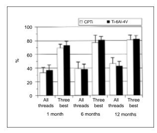
**Fig 3** Mean percentage of bone volume in the threads around the entire implant and in the three best consecutive threads in the cortical region. There were no statistically significant differences between the materials at any time of follow-up.
