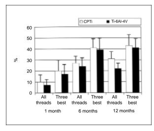
**Fig 2** Mean bone-metal contact around the entire implant and in the three best consecutive threads in the cortical region. There were no statistically significant differences between the materials at any time of follow-up.
