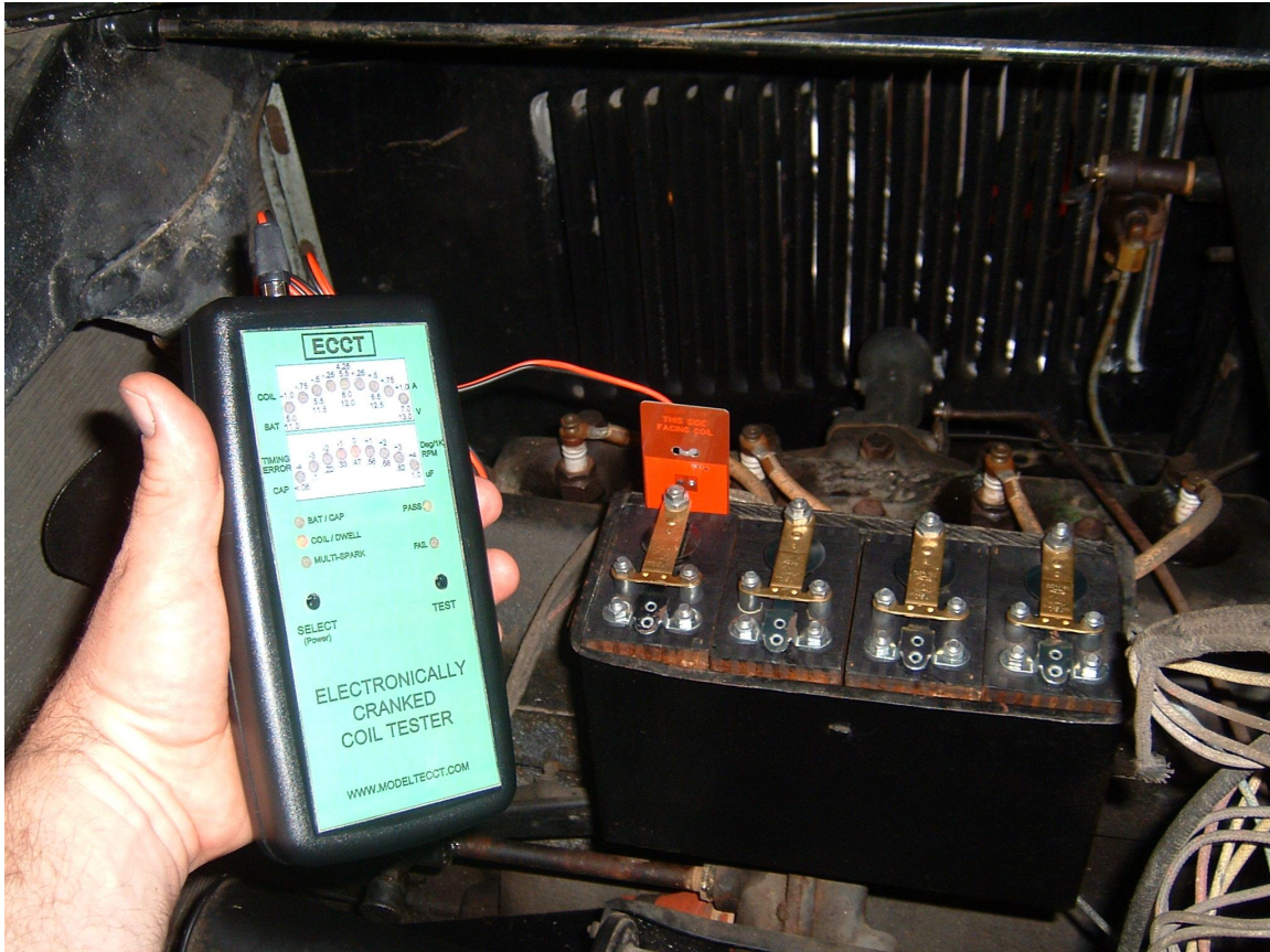
Figure 3 – The Electrically Cranked Coil Tester (ECCT) Prototype
