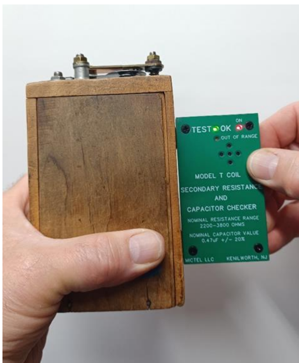
Figure 1 – Secondary Resistance Test
