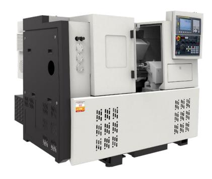
We have Ace, Bangalore make CNC turning machines. Size 200mm x 300mm, Chuck size 6 inches and 8 inches Quantity – 03 NOS.
