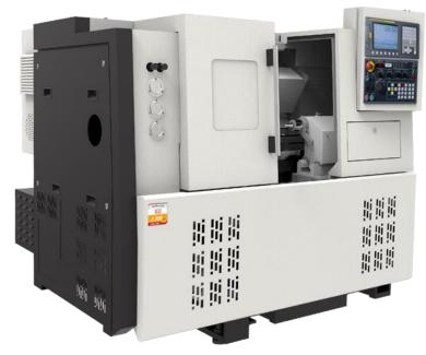
We have Ace, Bangalore make CNC turning machines. Size 200mm x 300mm, Chuck size 6 inches and 8 inches Quantity – 02 NOS. The accuracy obtained by the machines is 10 microns
