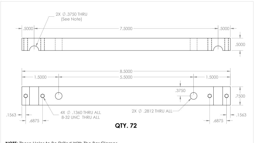
**NOTE:** These Holes to Be Drilled With The Bar Clamps Installed and a Copper Spacer Between The Bars.
