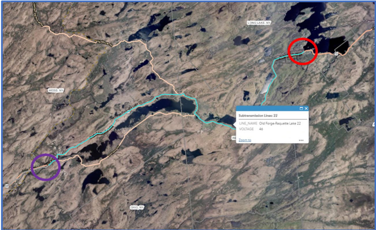
Figure 3: Old Forge - Raquette Lake 46kV line (light blue) that runs along State Route NY-28 highway. This line runs between Old Forge Substation (purple circle) and Racquette Lake Substation (red circle)
