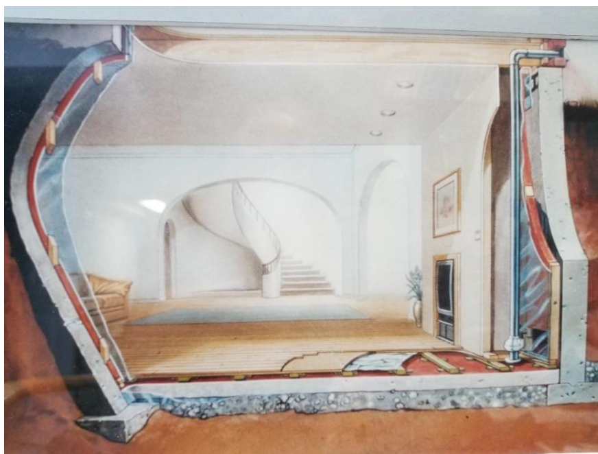
Figure 1 ECHO basement living space is healthy living space, doubling the available quality living space in bungalows and increasing it by a third in two story residences. Its wall and floor ventilation rate is an order of magnitude more effective than that of a heat recovery ventilator in eliminating basement microbial air pollutants. Most importantly, foundation leakage problems are permanently resolved without costly exterior digging.
