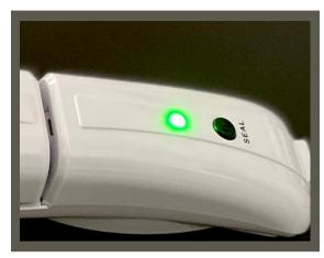
Push **SEAL** button once to begin sealing. When the LED blinks & turns off, sealing is complete.
