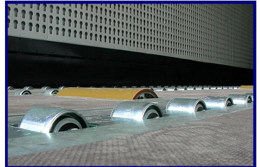
There is also a low height version available for installation within a restricted space such as the cramped area above the vehicle's chassis 5th wheel coupling or inside of the frame work of a floor mounted loading dock. The roller is fitted with a wear resistant urethane cover to prevent any damage to the
