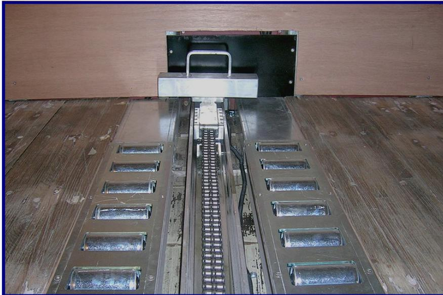
The Rollerbed Systems T-Bar Off-Loader is a vehicle mounted off-loading system aimed at those users carrying palletized loads such as empty food or beverage cans, glass bottles or finished products. The system is mounted flush within the floor of the trailer to maintain continuity with standard loading docks. The single chain drive unit is mounted centrally at the front bulkhead to provide a direct inline pull on the load.
