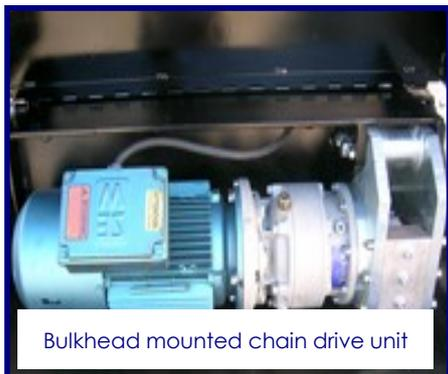
Bulkhead mounted chain drive unit
