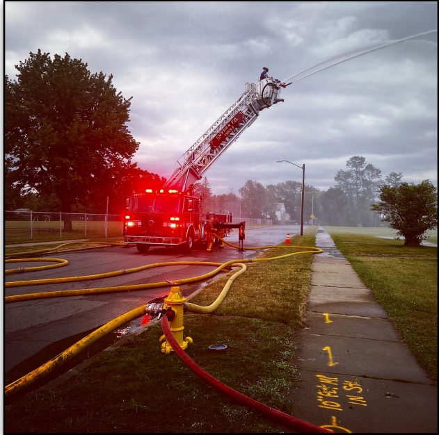
Truck 6 Flowing both Master Streams with 2" Tips Delivering Massive GPM. Flows possible because of Multiple Intakes.
