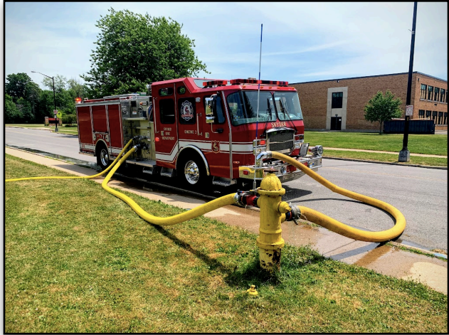
Engine on the Hydrant with Front Suction Connected and 4" LDH connected from the 2-1/2" Outlet to the Side Intake
