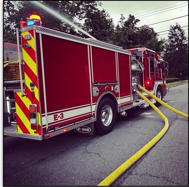
Engine Taking a Feed from the Hydrant and Supplying a 4" Feed off the Officer Side. In addition we utilized both 4" Intakes and the 4" Discharge off the Rear.
