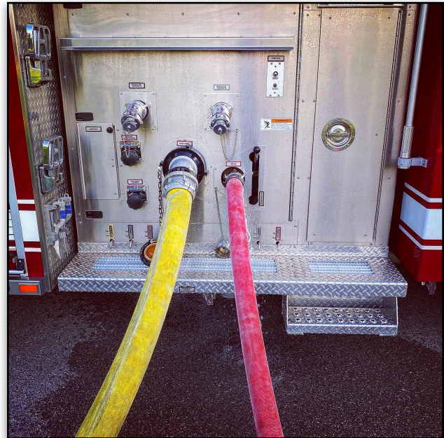
Engine Taking Multiple Feeds - 4" Side Intake and 2-1/2" Auxiliary Intake
