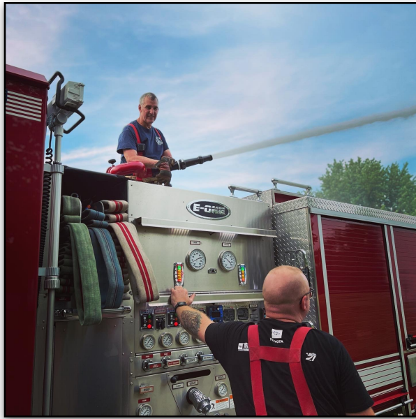
Flowing Over 800 Plus GPM on the Stang Nozzle with 1 3/4" Tip — Pumped at 80 PSI, but Volume of Water Made the Stream Possible.
