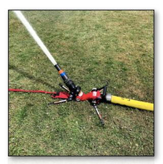
Consider the RAM appliance to apply a high volume of water (505 GPM).
