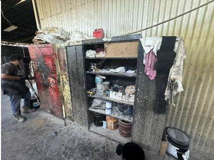
Improper storage of solvent contaminated rags
