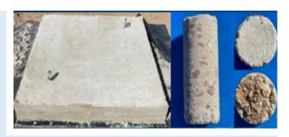
concrete soil additive mixed with soil. Above, a Slab and cores from the slab, mixed site soil with Pro-SealECCO alternate concrete additives and poured into a form achieving >3,800 psi.
