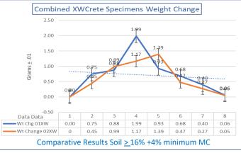
Wet Soils Moisture content (MC) Results: Water Expulsion = Hydrophobic/Anionic
