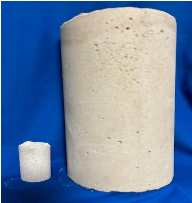
Site dirt treated with Pro-SealECCO Additive = alternate concrete
