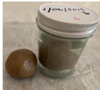
Image Left: Impermeable, Its hydrophobic this Specimen has been submerged since 2014. No water has penetrated the surface, and no breakdown has occurred.
