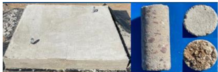
Above, Landfill Basin Soil Semi-Structurally Stabilized with type I cement characteristics.
