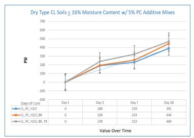
Compare Portland Cement (PC) stabilization psi (above) mixed with natural soils versus NanoCrete (NC) stabilization psi mixed with natural soils (below). NanoCrete stabilization clearly demonstrates significantly greater performance.
