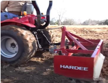
7. Back Drag or Box Blade for Initial Compression
