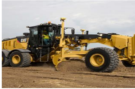
2. Grade To Slope and Drain
