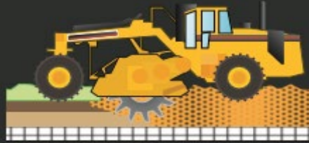
STEP TWO: Re-claim new road or recycle existing road to depth.
