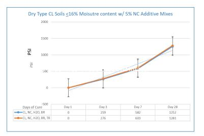
See graph (above) for dry soils increased PSI strength of ProSeal*ECCO*<sup>®</sup> NanoCrete stabilized soils structures and roads.
