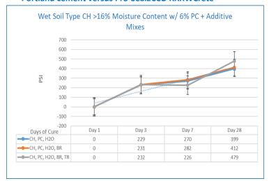
Compare Portland Cement stabilization (above) in wet soils versus XXXW NanoCrete stabilization for wet soils (below). XXXWNanoCrete stabilization demonstrates significantly greater performance
