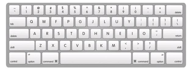
In addition to changing the position of the most frequently used character keys, Colemak remaps the Caps Lock key as a second Delete key. This change is one of the biggest innovations in Colemak. No one (aside from Internet trolls) uses the Caps Lock key on a regular basis, but it occupies prime real estate: it's an easy reach for the left-hand pinkie finger, and it's right next door to the A key on the home row.
