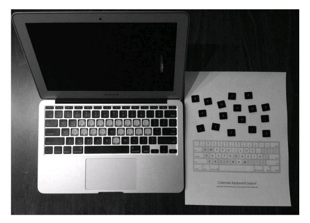
Using a small slotted screwdriver, I gently lifted the top right side of each key, inserted the tip of the screwdriver, then moved it down along the right edge of the key. Once the screwdriver gets to the middle of the key, the key pops off the keyboard's built-in "scissor" mechanism, which makes the key bounce back after it's pressed.
