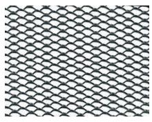
**Self-Furred Lath** is used extensively in exterior stucco and stone work over sheathing and as a plaster base over masonry walls. Self-furring dimples or embossed "V" grooves hold the lath minimum ¼" away from solid surfaces to aid in the keying of stucco to the lath. AMICO self-furred lath does not require additional self-furring mechanisms to function as required by ASTM C1063.
