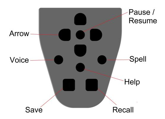
**Help Button:** This is the round button located in the center of the keypad. Press the help button together with any other button to hear a description of the button and its function. Press the button on its own to hear general help information.
