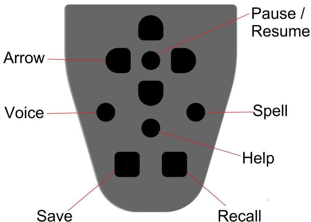
**Help Button:** This is the round button located in the center of the keypad. Press the help button together with any other button to hear a description of the button and its function. Press the button on its own to hear general help information.
