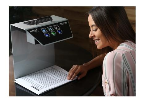
Step One - Remove unit from box and set the unit atop a sturdy surface upright with handle on top and the six pack of tactile controls facing the user. We suggest you take a moment to gently feel the entire unit from top handle to the rear of the unit and canvas your hands over the sides, the bottom, and the canopy that houses the six tactile controls. Note that there are three square controls stacked atop three round controls.
