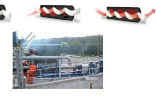
Applications for PC Pumps are so varied it is hard to list them all. Aside from being a positive displacement pump, some of the advantages of PC Pumps are repeatable flow rates (metering), ability to move solids, abrasives, sewage, sludge, grout, cement, etc.. PC Pumps also have the ability to pump heavy sour oil with high viscosities. The most common applications in the oil field are downhole artificial lift, surface oil transfer, slurry pumping, recycle and skim pumps.
