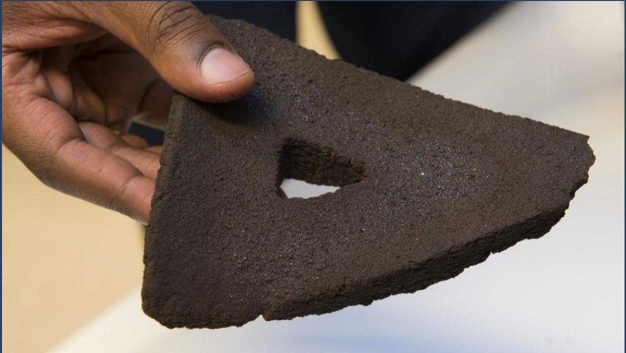
Figure 2_3D Printed Brick from Moondust using Focused Sunlight _© https://spacearchitect.org/portfolio-item/regolight-2/
