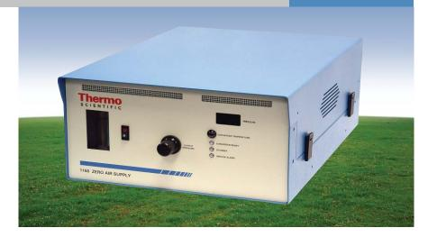
The Thermo Scientific Model 1160 Zero Air Supply is a source of ultra high purity zero air for analytical and process instrument needs. This modular unit can be configured for the removal of a variety of pollutant gases. Up to 20 liters per minute of clean dry air can be supplied at pressures up to 60 psig via a self-contained compressor.
