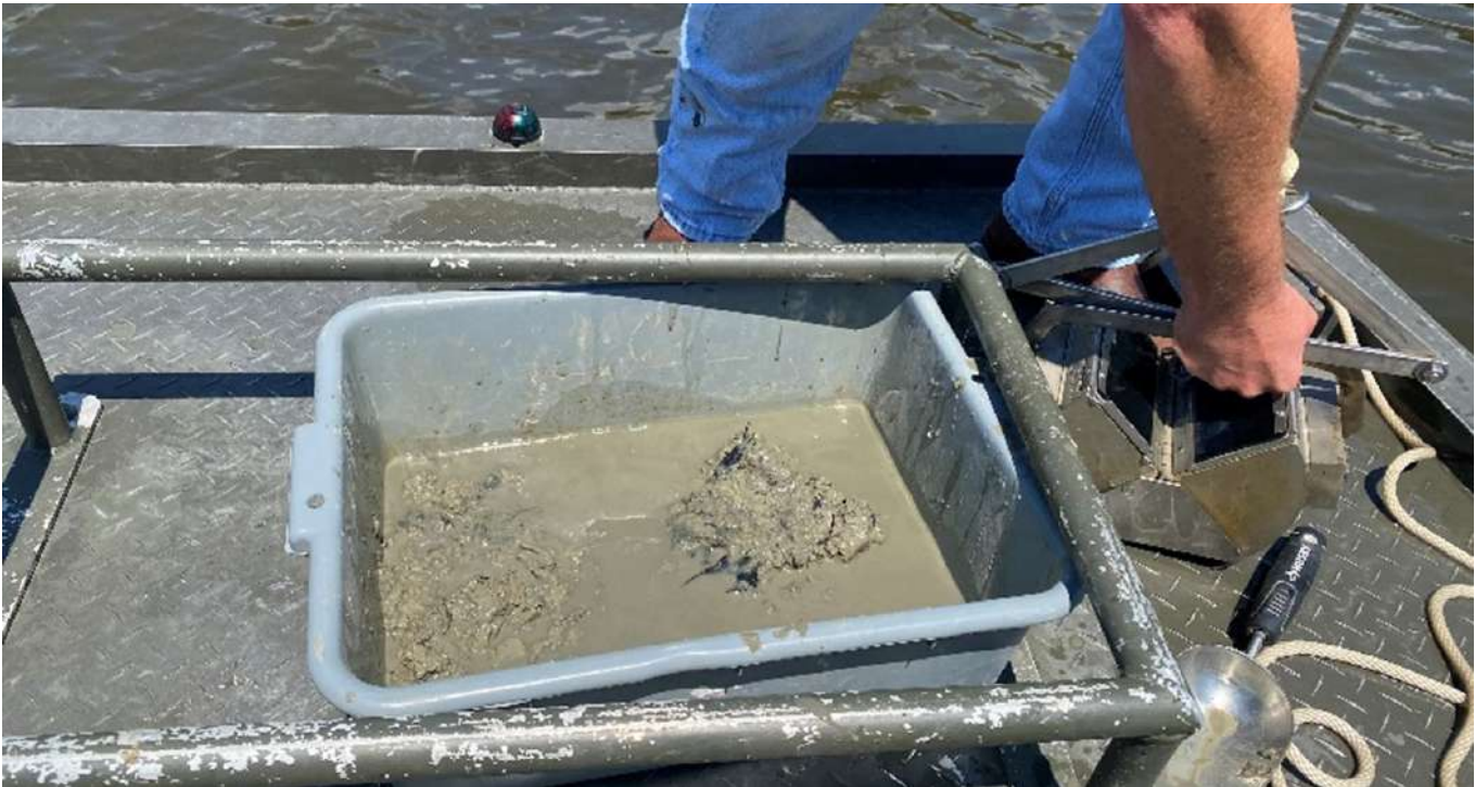
FIGURE 3-4: GRAB SAMPLER AND SEDIMENT SAMPLE TAKEN ON THE AMITE RIVER DIVERSION CANAL (PHOTO SOURCE: ARBC)
