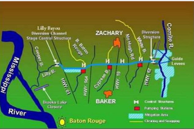
FIGURE 2-14: COMITE DIVERSION PROJECT SCHEMATIC MAP (PHOTO SOURCE: USACE)
