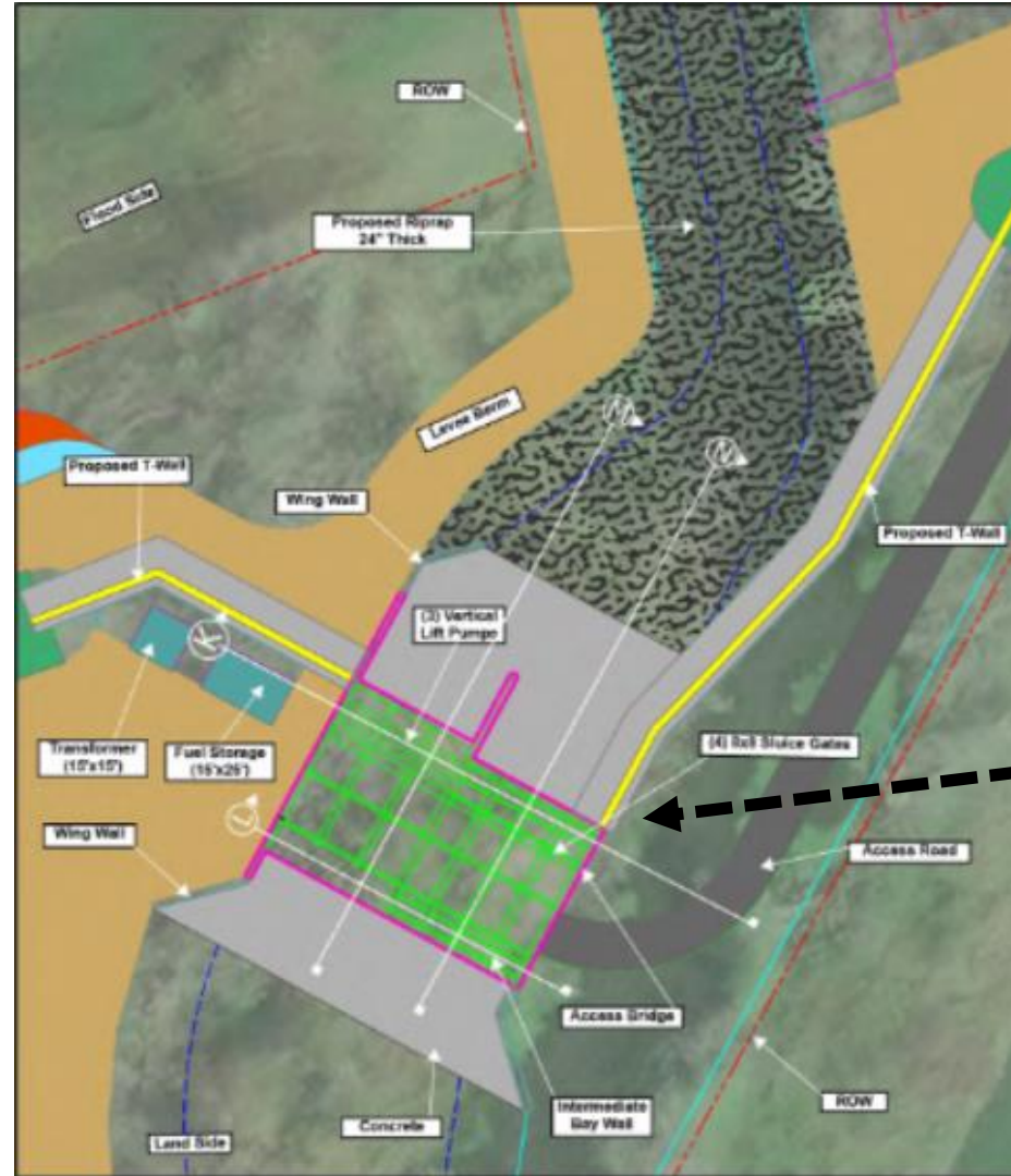
M-2 East Pump Station and Drainage Structure Plan View (from Permit Application)
