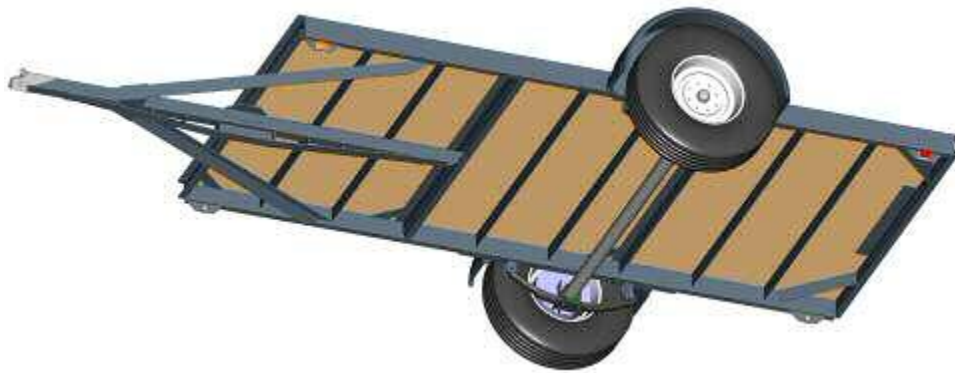
Tongue Stiffener Braces Under the 6x12 Trailer. Others Trailers Similar.
