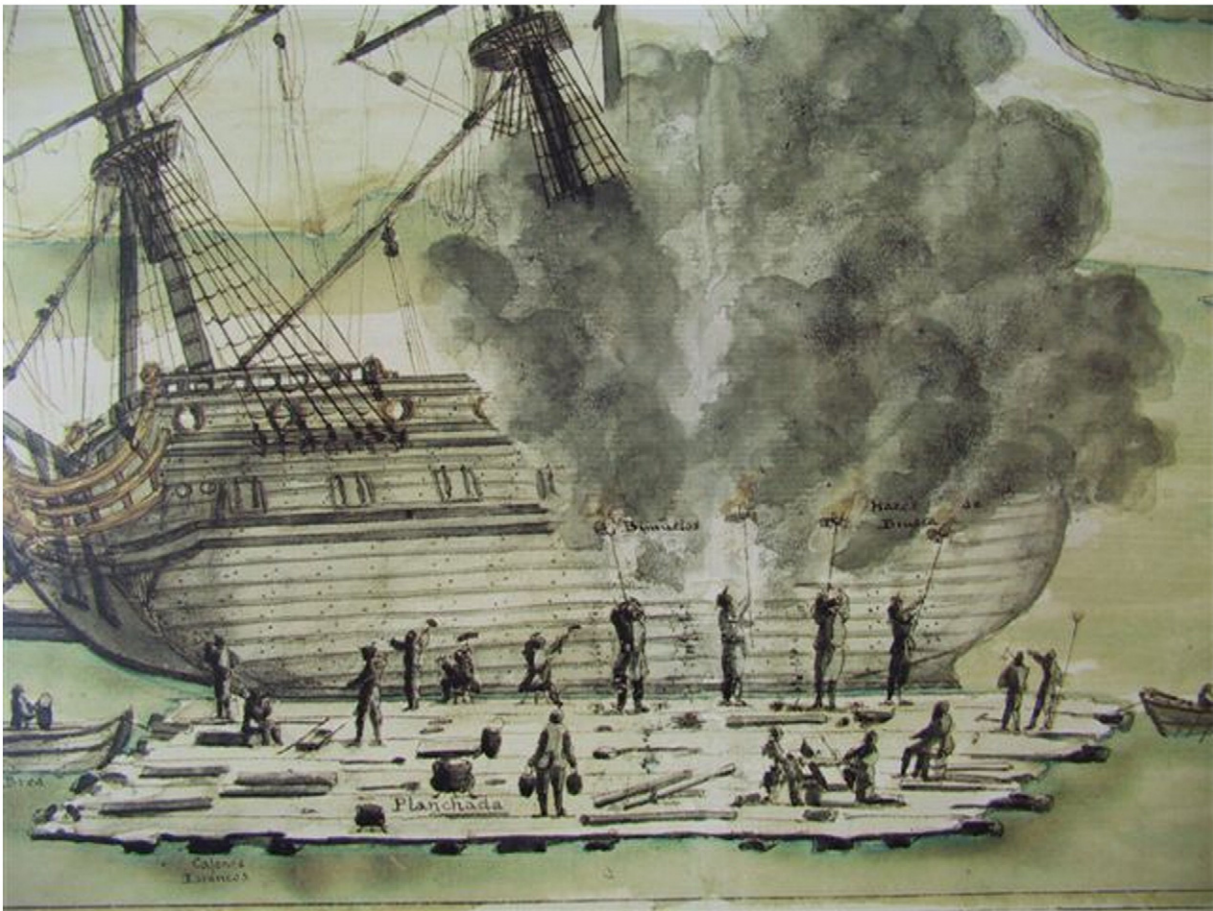
Fig. 4. Repair works and caulking of a wooden ship (Copyright: Museo Naval de Madrid).
