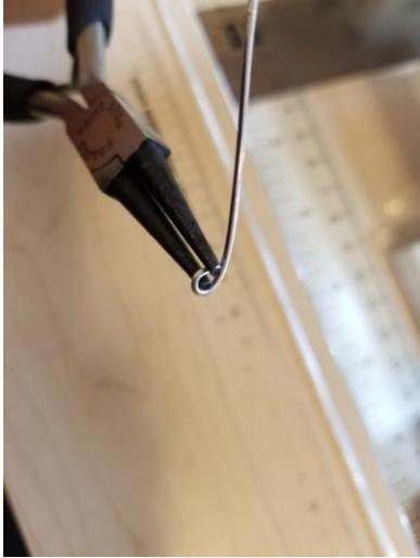
Use small needle nose pliers to form both ends of the wire into a small loop.
