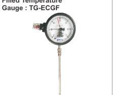
Nominal size: 100 and 150 mm Compliance to latest EN13190 Std. ranges: -20°C to 400°C Overload capacity 110 % of FSD Protection to IP67
