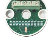
Solder jumpers for : Span, Zero, Upscale/down Scale
