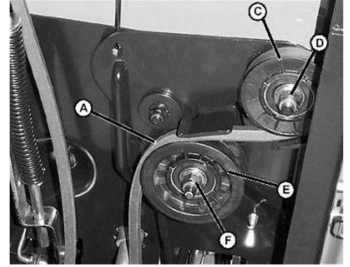
5.Remove mower belt. 6.Clean top of mower deck and sheaves. 7.Inspect belt for wear or damage; replace as necessary. 8.Install belt on mower deck and fasten with six cap screws. Install mower deck and adjust mower engagement rod, if necessary. Move lift lever to transport position. May 11, · Im looking for a drive belt diagram for a Deere LT - Answered by a verified Technician Im looking for a drive belt diagram for a John Deere LT Show More.
