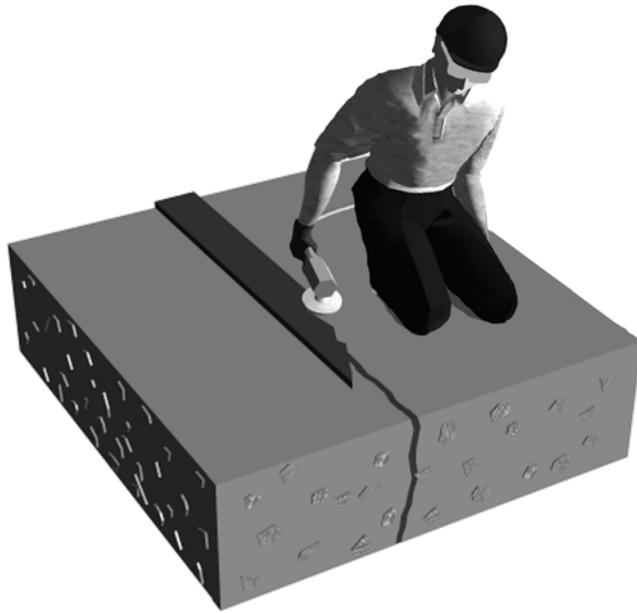
Fig. 6—Remove seal cap.
