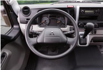
An infinitely adjustable steering wheel and dash-mounted shifter give drivers more control, while instruments and displays are always within easy reach or view. By moving the shifter off the floor, we create more leg room and easier access for passengers.
