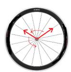
b) Linear speed describes the distance covered by a point on the circumference path of the rotating item.
