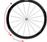
Therefore, the linear speed of the wheel is approximately 32,672 inches/minute or 2723 feet/minute
