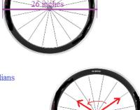
b) Linear speed describes the distance covered by a point on the circumference path of the rotating item.
