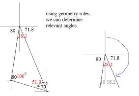
Note: Using horizontal and vertical axes maintain consistent bearings and help determine angle measurements.
