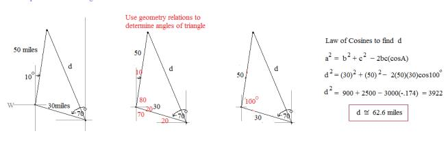
Step 3: Fill in triangle with angle measurements and find bearing
