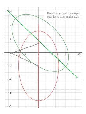
Find the equation of the ellipse after it is rotated 45 degrees counterclockwise
