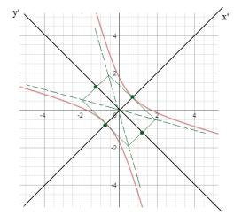
vertex: (1, 0) and (-1, 0) on the x'y'-coordinate plane.. foci: (2, 0) and (-2, 0) on the x'y'-coordinate plane.. asymptotes:  $y' = \sqrt{3} x'$  and  $y' = -\sqrt{3} x'$
