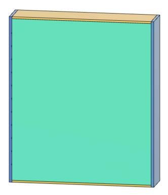
Cut 14-1/8" x 2-1/4" piece of 1/8" hardboard for center divider.
