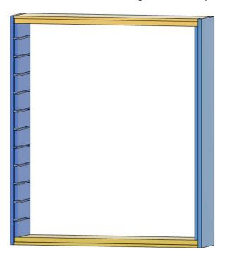
Cut 12-5/8" x 14-3/4" piece of 1/8" hardboard for the back.
