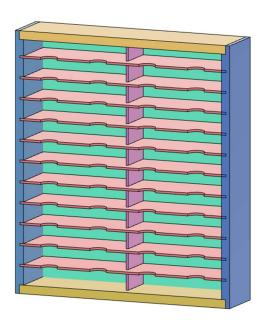
Cut Two pieces of  $\frac{12}{2}$  plywood to 12-5/8" x 2-15/16" for the top and bottom.
