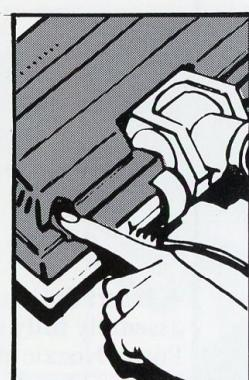
5. Replace bottom plate. Be sure front edge is in groove provided. Tighten screws securely. Replace wand. Replug cord (in sheath). Press RESET button.
